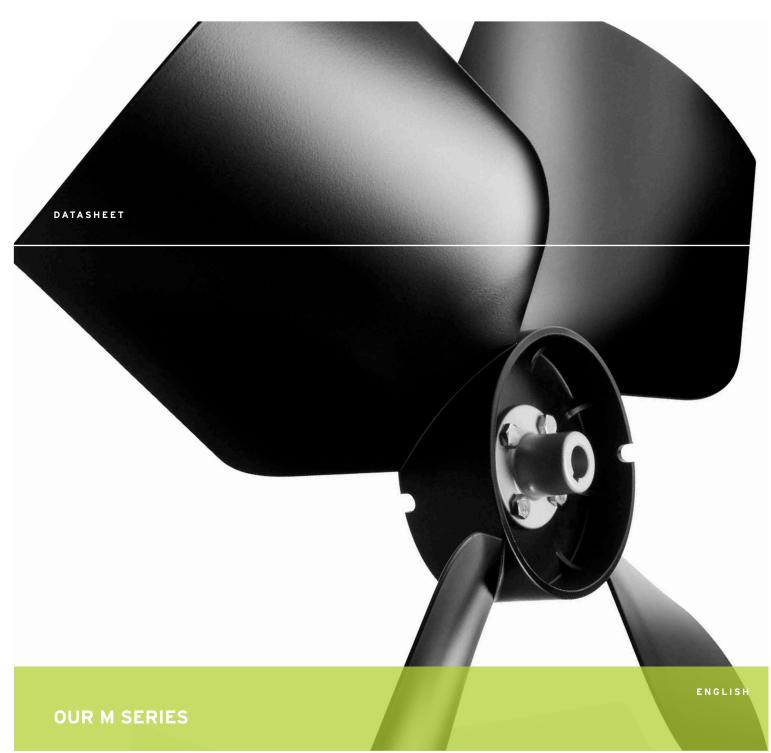
The M series covers diameters from 285mm up to 508mm. The M series is engineered to meet the demands of smaller heat exchangers such as oil coolers, air-cooled condensers and dry coolers. With fan blades of glass reinforced polyamide this axial fan can also be used in low temperature evaporator applications.
