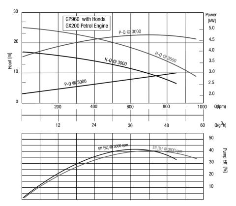
Please note: All tests carried out with potable water @ ambient air temperature.
