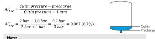
$AF_{sup}=0$  if cut-in pressure  $\geq$  precharge
