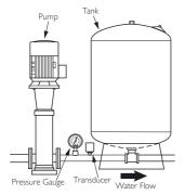
Fig. 1.4-6 Booster Pump w/ Tank
