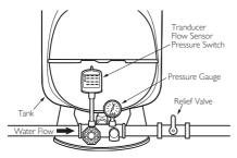
Fig. 1.4-1 Tank Installation with Accessories
