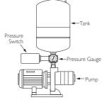
Fig. 1.4-5 Booster Pump w/ Inline Tank
