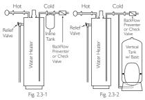
Thermal expansion inline tanks are designed to be supported by system piping and should be connected to the system piping using a "T" connection (See Fig. 2.3-1). Optional wall mounting brackets are also available for increased support (check with your local GWS dealer for more information). Vertical tanks with base are designed to be self-supporting and should be connected to the system with additional piping (See Fig. 2.3-2).
